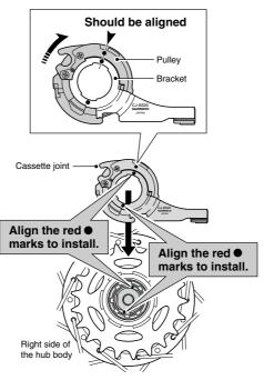
Secure the cassette joint to the hub with the cassette joint fixing ring. When installing the cassette joint fixing ring, align the yellow ● mark with the yellow ● mark on the cassette joint pulley, and then turn the cassette joint fixing ring 45° clockwise
