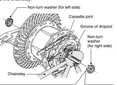
Use whichever non-turn washers match the shape of the dropouts. Different non-turn washers are used at the left and right sides.
