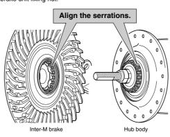
Refer to the Technical Service Instructions for the Inter-M brake for details on installing the Inter-M brake.
