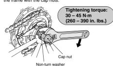
When installing a part such as a mudguard stay to the hub axle, install in the order shown in the
